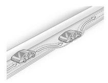
If the level of the shoulder is only slightly below the pavement, recovery should be fairly easy. Ease off the accelerator and then, if there is nothing in the way, steer so that the vehicle straddles the edge of the pavement. Turn the steering wheel 8 to 13 cm (3 to 5 in), about one-eighth turn, until the right front tire contacts the pavement edge. Then turn the steering wheel to go straight down the roadway.
